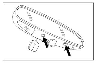
Push the buttons on the bottom of the mirror to turn the reading lamps on and off.
